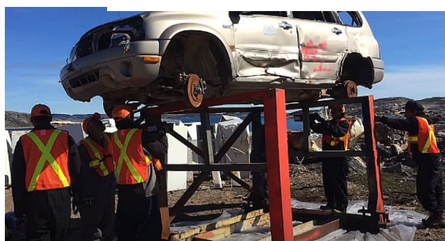
Figure 4. ELV placed on top of a sturdy metal frame
