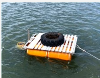
Figure 2: "Seabin mounted to a pontoon and anchored down to a fixed location at the University of the South Pacific, Marine Studies campus jetty". Source: Paris, Kwaoga, & Chintaka (2022).
