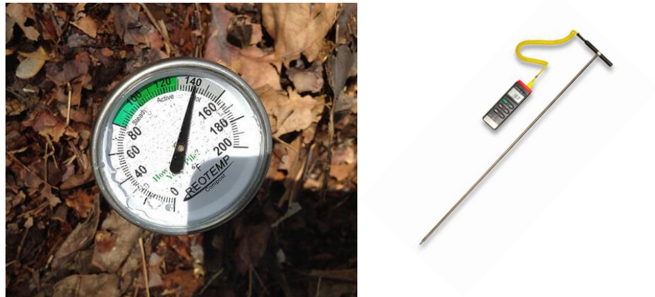
Figure 2: Temperature probes of varying length (30 – 150 cm) are available with dial readout (left) or digital display (right)
