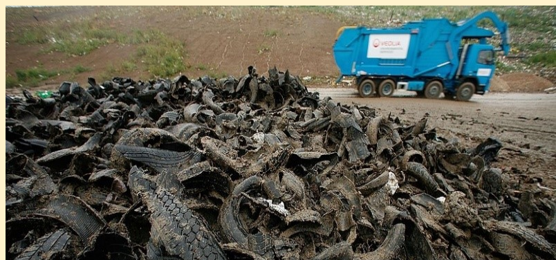
Figure 9: Shredded ELT as Landfill cover
